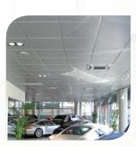
Standard systems that can be adapted to all types of ceiling design: tiles are installed on a T grid and can easily be removed by simply lifting the tile.
