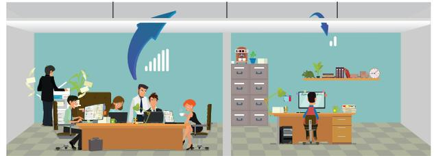
The sound insulation performance of a suspended ceiling can be defined by its ability to reduce the propagation of sound waves between adjacent rooms sharing the same plenum. It is expressed in decibels.
